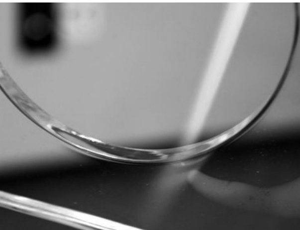
FLAME POLISHING OF ACRYLIC EDGE
